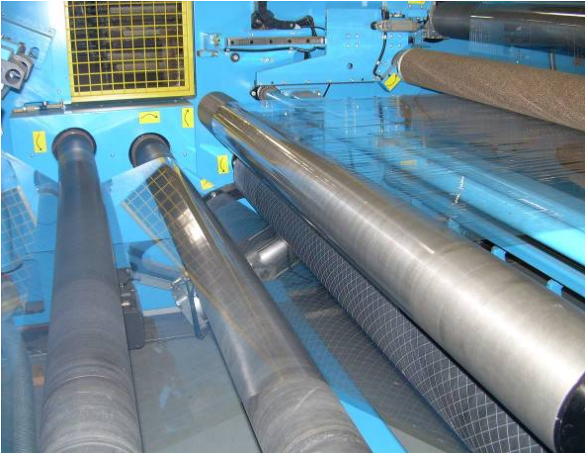
Photo: 8-micron thick Halar® ECTFE film being extruded on a 72-inch wide die at Ajedium.
